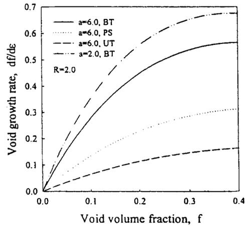
Fig. 4 Variation of void growth rate with void volume fraction for  $a=2.0, 6.0$  and  $R=2.0$
