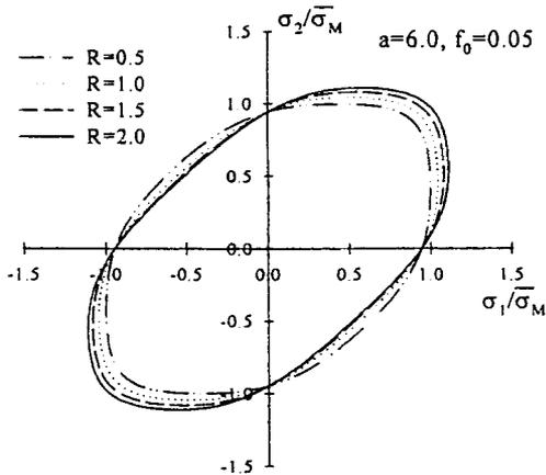
Fig. 3 Effect of plastic anisotropy parameter on the yield loci for  $a=6.0$  and  $f_0=0.05$
